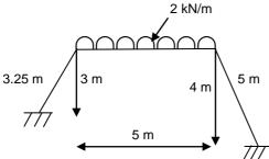
2 Analyze the portal frame shown in figure below by strain energy method.
