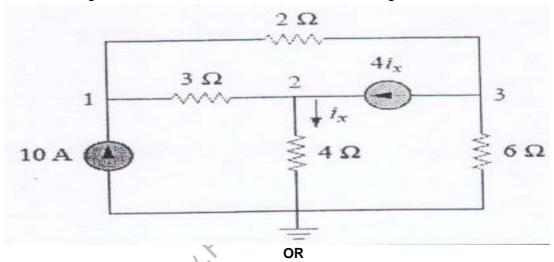
7 Using Mesh analysis determine  $i_1$ ,  $i_2$ ,  $i_3$  for the circuit shown in figure below.
