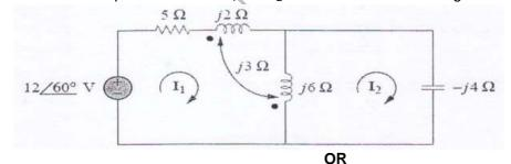
3 Determine the currents  $I_1$  and  $I_2$  for the circuit shown in figure below.
