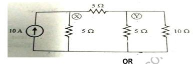
9 For the network shown in figure below, write tie set matrix, write equilibrium equations and obtain the loop currents using network topology.
