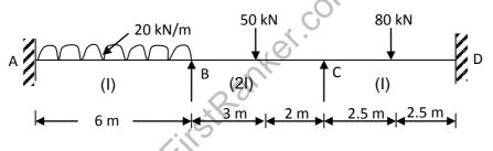
A continuous beam ABCD is loaded as shown in figure below. The support B sinks by 10 mm below the levels of A, C and D. Assume E = 200 GPa and I =  $32 \times 10^6$  mm<sup>4</sup> for all the members. Use moment distribution method. Draw the bending moment diagram.
