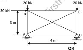
A braced cantilever truss is loaded as shown in figure below. All the members are of the same material and have the same cross sectional area. Find the axial force in the member AD by strain energy method.
