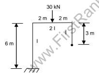
4 Analyze the portal frame shown in figure below, using moment distribution method. Draw the BMD.
