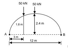
3 Analyze the portal frame shown in figure using slope deflection method.
