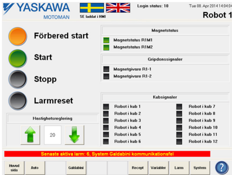
Figure 1.7: Example of the main status page from a Yaskawa HMI developed in Beckhoff's TwinCAT 2
