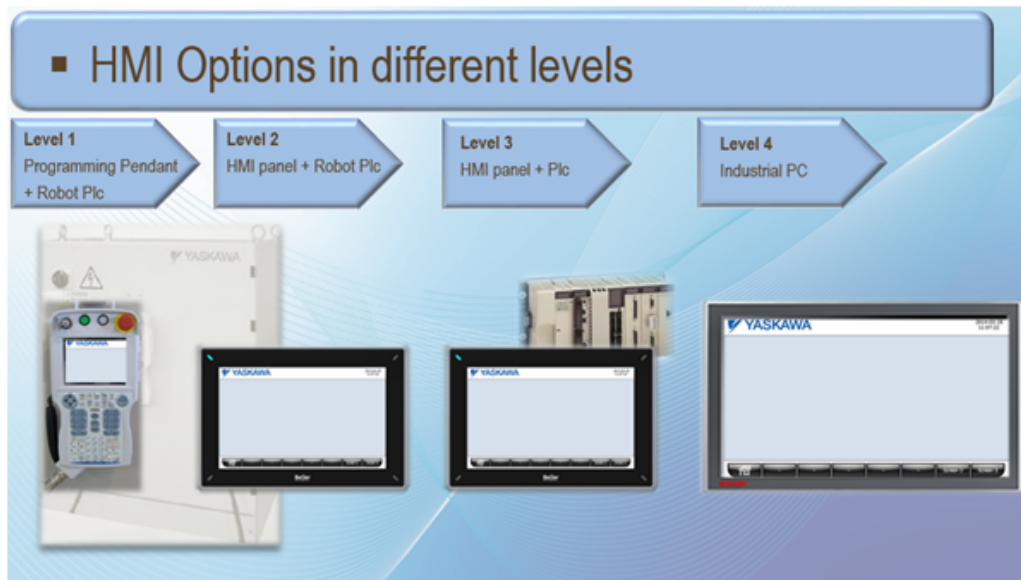
Figure 1.3: Different platforms for HMI presentation, the first alternative is a programming pendant, or teach box. The two following ones are HMI operation panels and the last one is a regular screen connected to a PC
