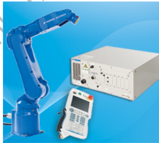
(b) A robot, its teach box and control system
