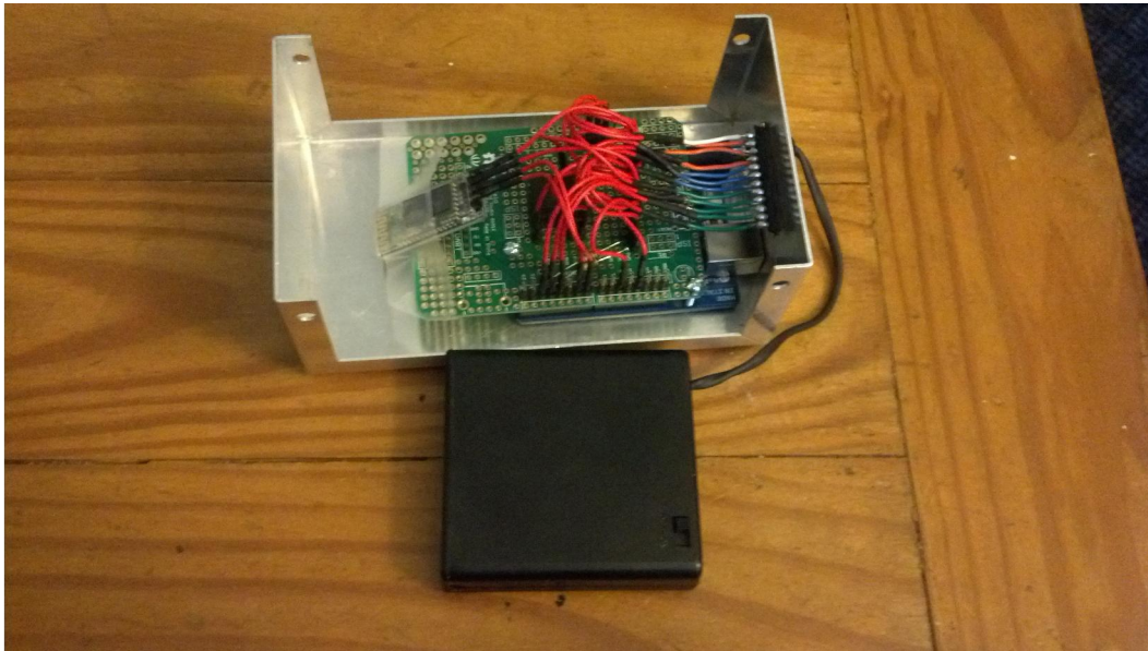
Figure 16: The Inside of the final enclosure, featuring the custom made Arduino Uno shield, battery pack with power switch, and the female header pin array.
