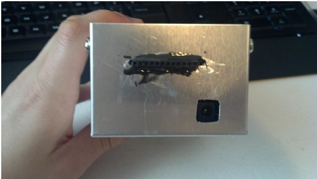
Figure 17: The outside of the final enclosure, featuring the plug for the battery pack and the female header pin array attached to the enclosure with J.B. Weld.
