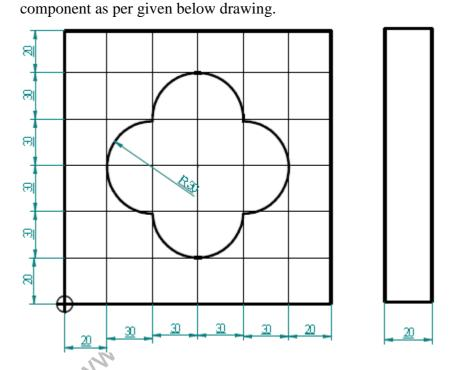
All Dimensions are in mm. Assume suitable data if necessary.
