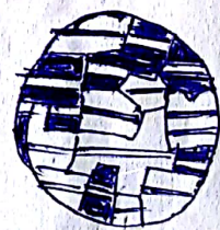
Structure of cartridge brass
