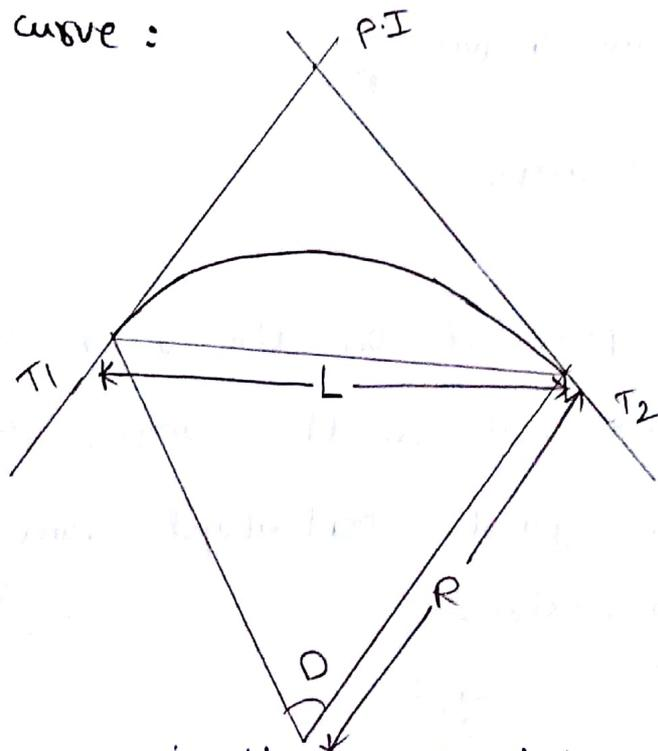
Degree of curve is the angle between the two tangents and the ending of the  $T_1$ , and  $T_2$  which are the starting and the ending of the curve.
