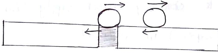
Here the creep is mainly due to dragging of wheels on the rails against its movement.
