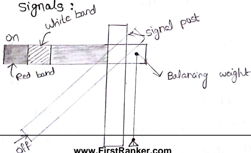
Semaphore signals are the mechanically operated signals in this a signal post which is attached by the horizontal lever.
