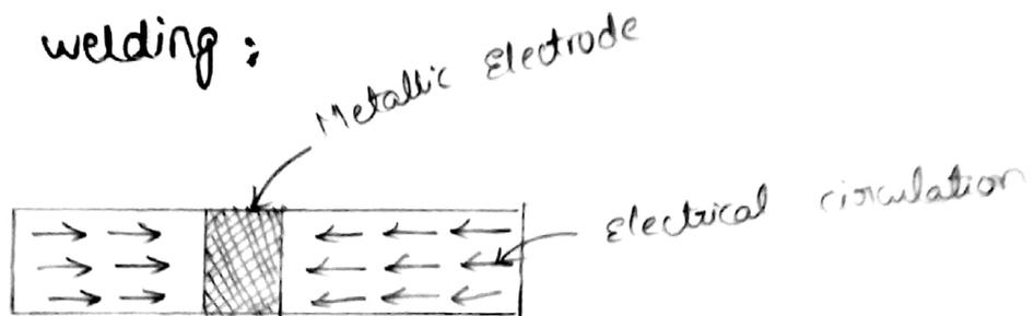
In this method an metallic electrode is placed between the two rails then electrical supply is applied from the both ends of the rails upon the metallic electrode is melted
