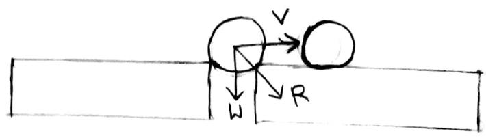
In this the creep mainly occurs due to self weight of the wheel (W)
