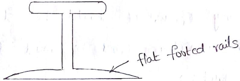
In this the foot of the rail much flatter than the bull headed rail. This flat footed rail is used for easy joining of sleeper and the rails.
