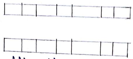
In this the joints are inner rail and outer rails are parallel to the each other and they should be in square shape.
