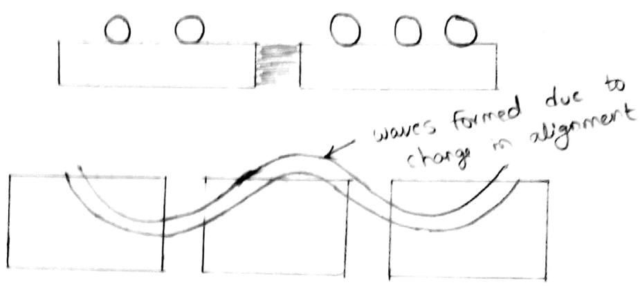
In this the creep is mainly due to the wave action at rail joints, bridges, level crossings intersections of joint junctions.
