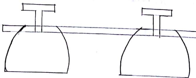
These sleepers are in the shape of pot. on the inverted pot the base of the rail is connected by using chairs
