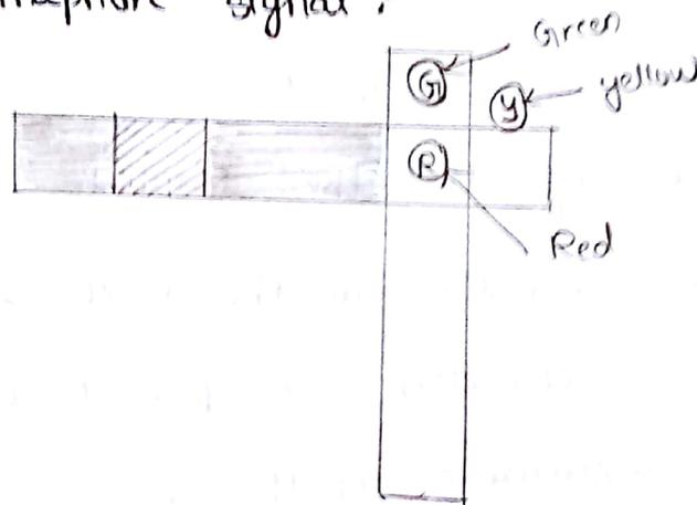
Warner semaphore signals are the advanced to the semaphore signals which include lever with the high intensified lights.
