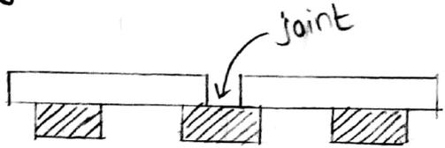
In this the rails are joined by using fillet material. that should be supported by sleepers.
