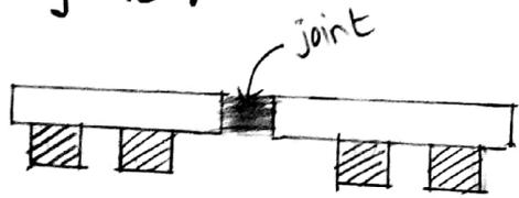
In this joint is filled with suspended material (melted)
