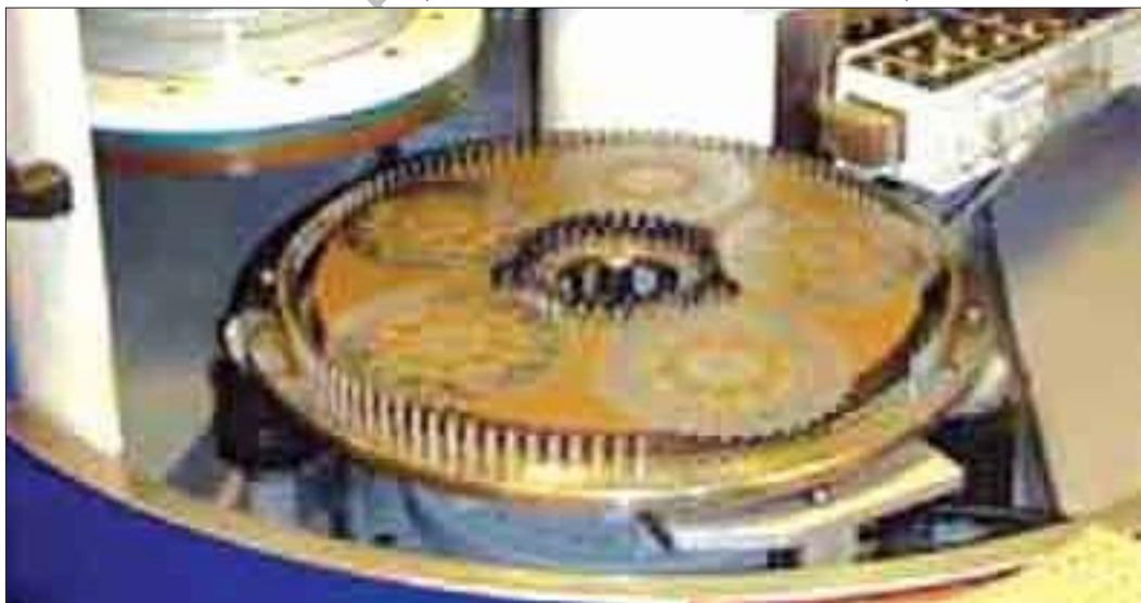
Lapping is a surface finishing process for finishing gears, etc.
