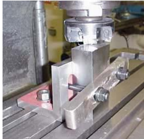
Figure 10: Angle plate being used to machine
