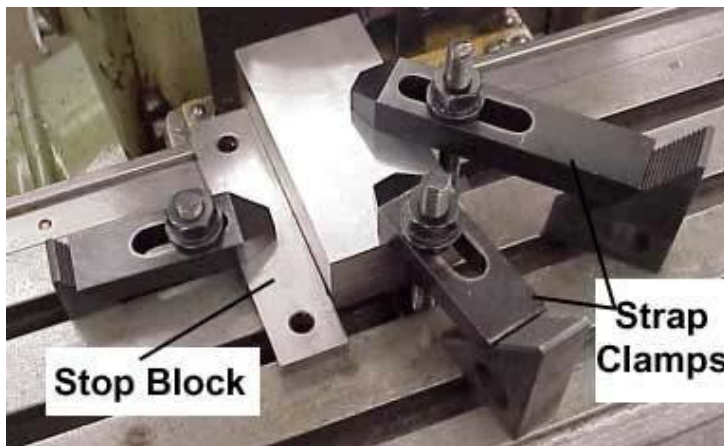
Figure 11: Direct Clamping using strap clamps-Notice the stop block. It is used to align the work as well as prevent the part from slipping.
