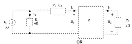
11 Obtain the hybrid parameters for the two port network shown in figure below.
