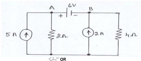
9 Calculate the value of R which will absorb maximum power from the circuit of given below. Also find the value of maximum power.
