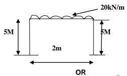
7 Analyse the frame as shown in fig below using Kani's method and sketch the bending moment diagram?
