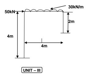
6 Analyse the frame as shown in fig below using Kani's method and sketch the bending moment diagram?
