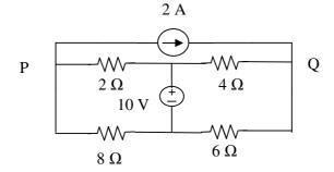
3. a) Draw the graph of the network shown in below figure and write down the tie-set (7M) matrix.
