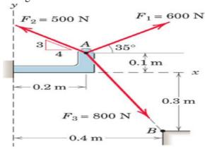
b) For the beam, reduce the system of forces shown in below figure to (a) an equivalent force-couple system at A, (b) an equivalent force couple system at B.
