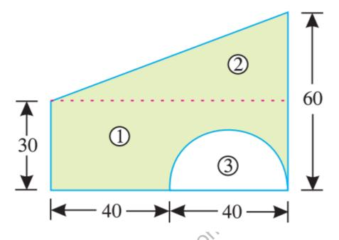
Find the moment of inertia of the section as shown in the fig about centroidal axis [16M] XX perpendicular to the web.
