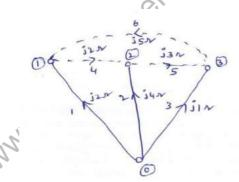
3 The power system network is as shown below; obtain V<sub>3</sub> using G-S method after first [16M] iteration. The impedance values in p.u indicted in the network.
