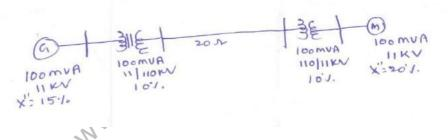
The synchronous generator is operating at its rated MVA at 0.95 lagging p.f and at rated voltage. A 3-phse short circuit occurs at bus A, calculate the p.u value of (i) subtransient fault current, (ii) subtransient generator and motor currents. Neglect pre fault current. Also compute (iii) subtransient generator and motor currents including the effect of pre fault currents.
