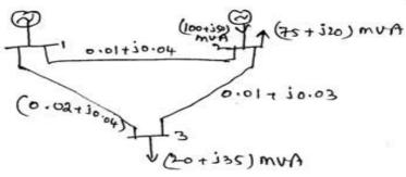
By using N-R method at the end of first iteration, determine the voltage magnitude and phase angle at buses 2 and 3.
