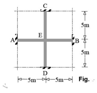
5. Derive Element stiffness matrix for Beam element as shown in fig
