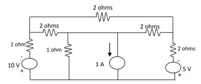
For the above network, draw (i) Graph. (ii) Tree. (iii) Dual network and also write down the procedure to draw dual network.
