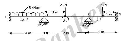
7 Analyze the continuous beam shown below using flexibility matrix method.
