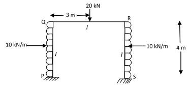
6 Analyze the beam shown by Kani's method. Draw SFD, BMD and elastic curve. Find the distance of points of contra flexure from supports
